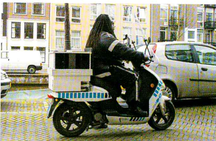
BELOW: SCANaCAR's equipment now fits into a small hatchback car with cameras and other sensors replacing the rear side windows LEFT: A lower specification system fits onto the back of a scooter
