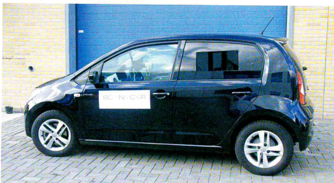
BELOW: SCANaCAR's equipment now fits into a small hatchback car with cameras and other sensors replacing the rear side windows LEFT: A lower specification system fits onto the back of a scooter
